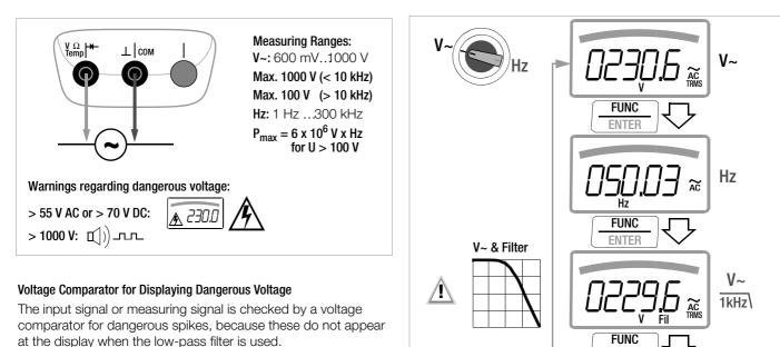
At voltages of greater than 55 V AC or 70 V DC, a danger symbol appears at the display:
