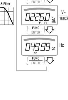
5.1.3 Alternating Voltage and Frequency Measurement V AC and Hz with Selectable Low-Pass Filter (METRAHIT EXTRA, METRAHIT ETECH and METRAHIT ESPECIAL only)
